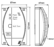
The detector and the gas stove should be placed in the same room. The detector should be mounted within 30cm to the floor. The detector should be within 1.5m  $\sim$  4m to the gas resource or the gas stove.
