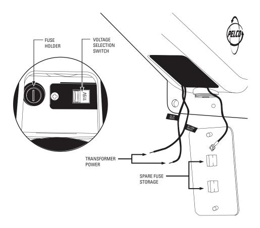
Figure 2. Voltage Selection Switch and Fuse Holder Location
