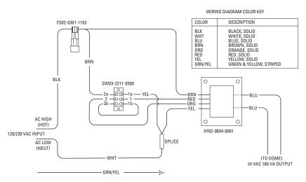
Figure 3. IWM24 Wiring
