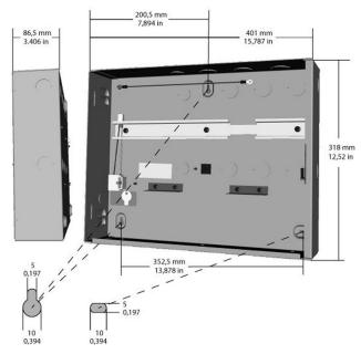
The enclosure is designed for installing an AMC2, a power supply (AMC PBC60) and two batteries.
