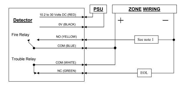
Note 1 – This component is the Fire Resistor, and its value is specified by the Fire Control Panel Manufacturer. For US installations it is typically a short circuit.
