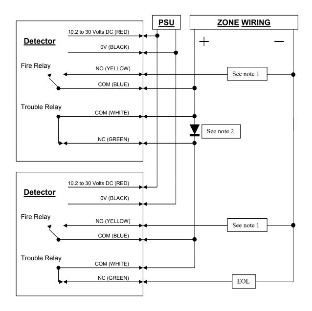
Note 1 – This component is the Fire Resistor, and its value is specified by the Fire Control Panel Manufacturer. For US installations it is typically a short circuit.
