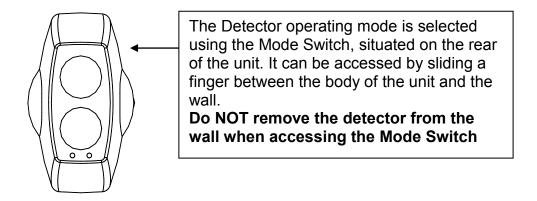
Select Prism Targeting Mode by moving the Mode Switch to the upper position.
