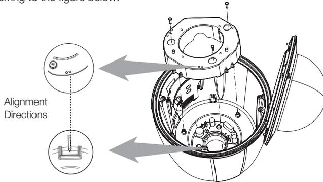
※ The lower bracket is exclusively for use with the SCP-3430 Series/SNP-5300 Series.
