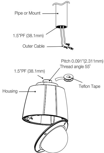
3. Install onto the pipe by turning the housing in a clockwise direction while referring to the figure below.
