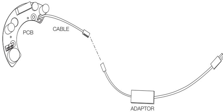
6. After inserting the external camera cable to the housing, connect to the corresponding jack on the adaptor.
