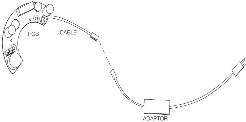
5. After connecting the camera adaptor and inner cable while referring to the installation manual, install the camera onto the housing and check if the adaptor hook is fastened properly onto the camera.
