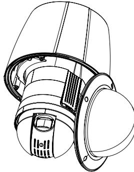
※ Remove the dome cover of the camera and install it onto the housing.
