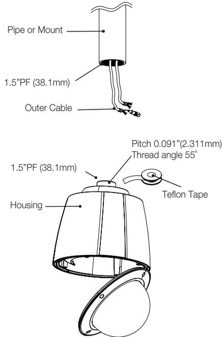
4. Install on the pipe by turning the housing in a clockwise direction, referring to the figure below.
