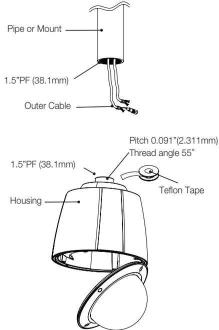
4. Install onto the pipe by turning the housing in a clockwise direction while referring to the figure below.
