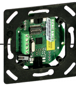
2 DG module BUS-2/BUS-1, f.m.
