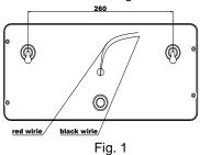
XT1 (red): connect to positive "+" of 24VDC or terminal R of the gas extinguishing control panel.
