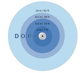
When mounted at a height of 3 m (10 ft) the 180° version of the camera has the following coverage radius for the four levels:
