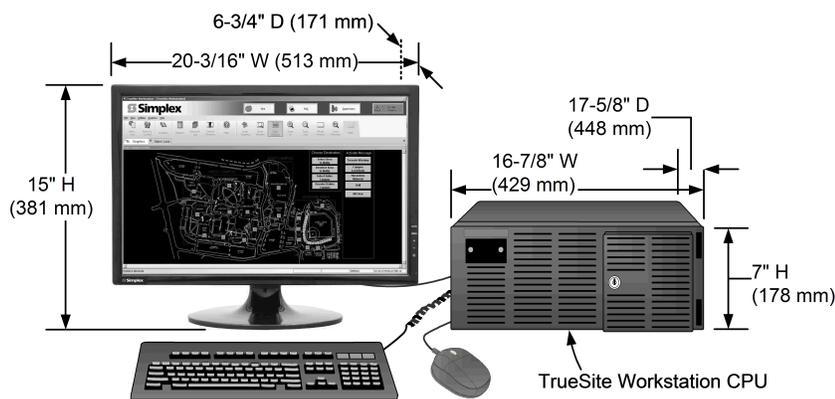
Figure 10: Hardware reference with 21.5" desktop monitor
