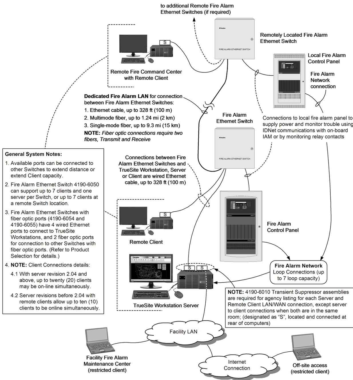
**Note:** The TrueSite Workstation PC has 2 Ethernet ports. On ES Net networks, the ES Net NIC connection uses (1) Ethernet port leaving (1) Ethernet port available for a connection to either an agency listed (dedicated) Fire Alarm LAN or a customer's LAN (not both). Refer to data sheet **S4190-0018** for additional information on Fire Alarm Network Ethernet Switches.
