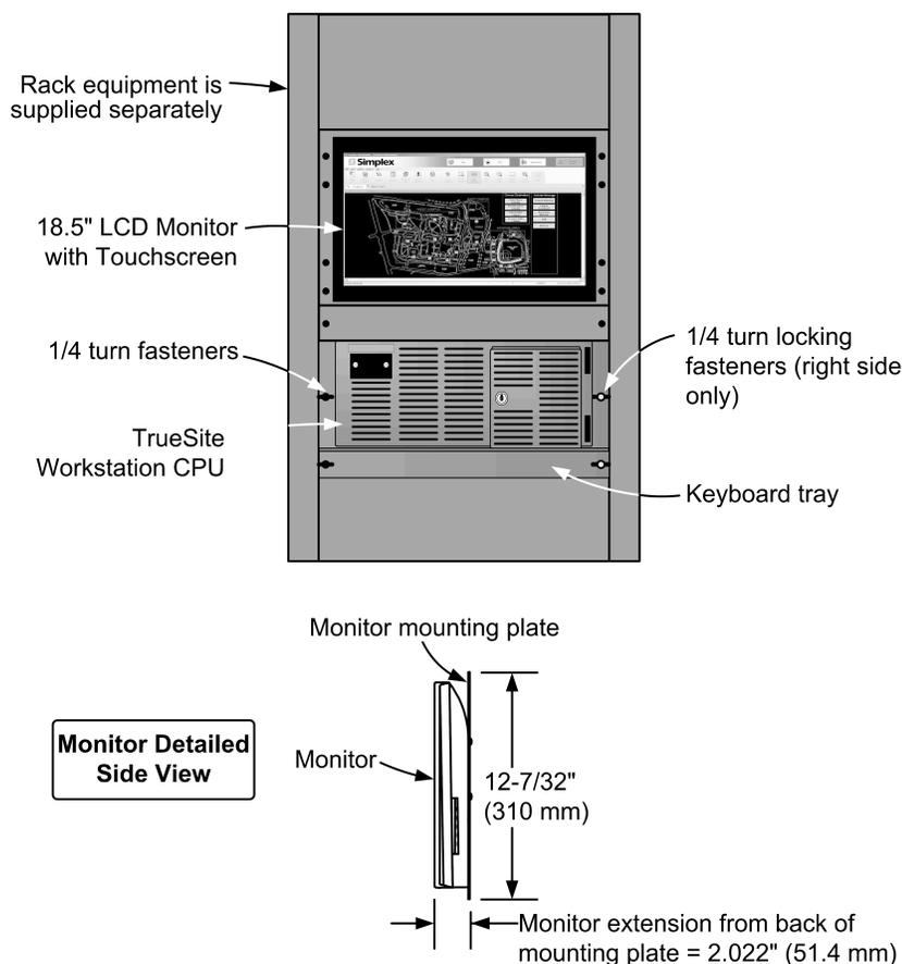
Figure 11: Rack mount hardware reference with 18.5" monitor
