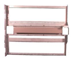
The MAP Hinged Mounting Plate (ICP-MAP0025) holds up to six modules and fits inside both the MAP Panel Enclosure and the MAP Expansion Enclosure. It is designed to hold up to four MAP LSN Gateways (ICP-MAP0010), one MAP DE Module (ICP-MAP0007), and one MAP Control Panel (ICP-MAP5000). The DE module and control panel space can also be used to hold two MAP Accessory Mounting Plates (ICP-MAP0020).
