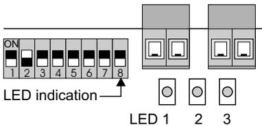
The DIP switch S8 is used to define the indication mode of the LEDs. (The DIP switch S8 is accepted when in operation.)
