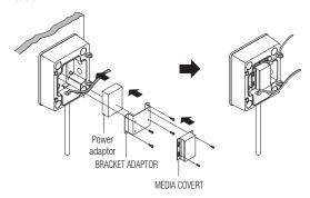
Pull the cable out through the door and wall mount and mount the door on the housing. (Return the locking lever to its original position and check that the hinge is properly attached to the housing.)
