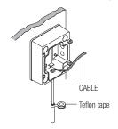
Install the power adaptor and media convert using the bracket adaptor, and connect the external cable.
