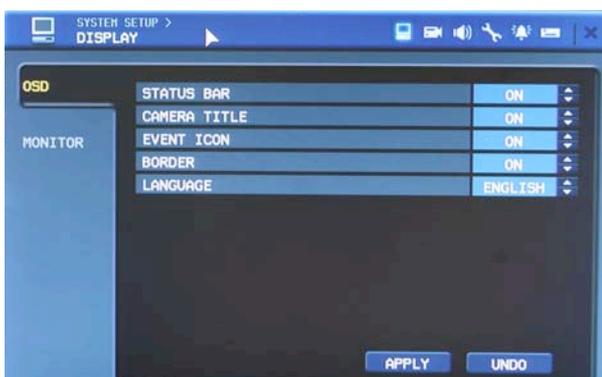
**STATUS BAR** : Turns the status bar at the bottom of the live display ON or OFF.
