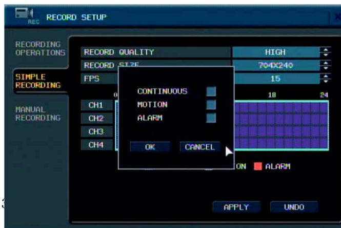
Click a single block to open the recording type menu. Click and Drag a block of times to configure multiple channels and times at once.
