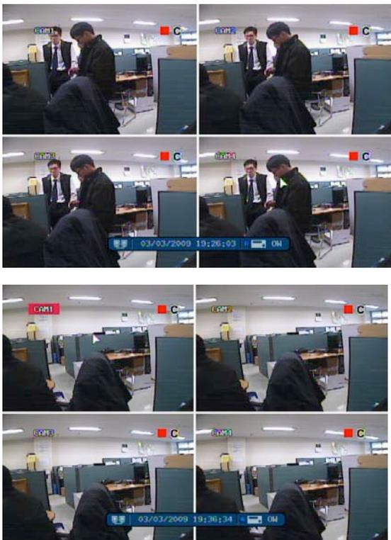
2 different display modes are supported by the 4 channel DVR. By repeatedly pressing the **DISPLAY** button, the operator can choose between single screen, 4 screen and basic sequence modes.
