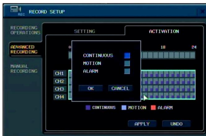
After selecting the channel and time, select the recording type.(Continuous, Motion and Alarm)
