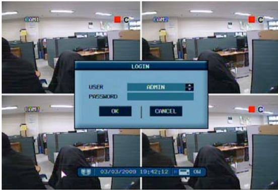
After startup diagnostics are complete, the operator must logon to the system. The default user name is 'ADMIN'. the default password of '1234' and press the **ENTER** button.
