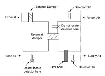
**Additional Information**. Refer to NFPA 90A, Standard for the Installation of Air Conditioning and Ventilating Systems; NFPA 72, the National Fire Alarm and Signaling Code; and the NEMA Guide for Proper Use of Smoke Detectors in Duct Applications, and Installation Instructions 574-776.
