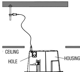
5. Push the **HOUSING** inside the **CEILING** through the **CEILING** hole, and tighten the **SCREWS** (x2) clockwise to fix the **HOUSING** on the **CEILING**.
