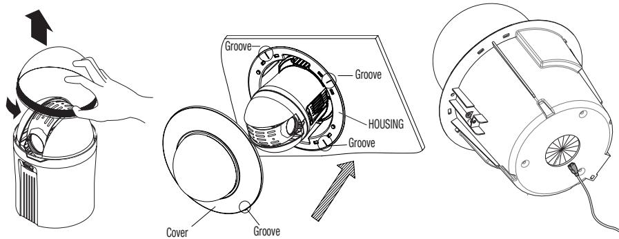
※ When working on the network PTZ camera, arrange the network cables through the bottom hole of the HOUSING.
