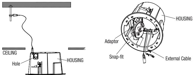
6. Push the **HOUSING** inside the **CEILING** through the **CEILING** hole, and tighten the **SCREWS** (x2) clockwise to fix the **HOUSING** on the **CEILING**.
