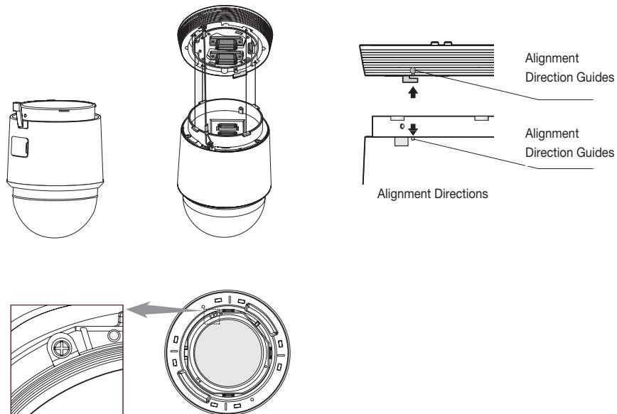
9. Remove the dome cover from the camera, and install the **cover** onto the **HOUSING**.
