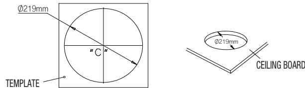
2. See the figure below to fix the **INSTALL BASE** that is provided as a camera accessory.
