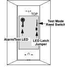
powering the unit off and then on or by placing a magnet over the reed switch (can be done with cover in place). Placing a magnet over the reed switch when the unit is in the test mode will terminate the test.
