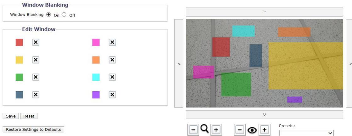
**FIGURE 3-27: WINDOW BLANKING ON**
