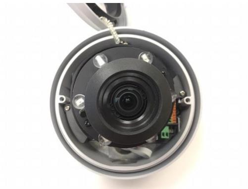
9. Adjust the angle of lens by pan and tilt by grasping the base.
