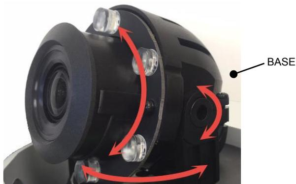
5. Tighten the locking screw to secure the camera module position.
