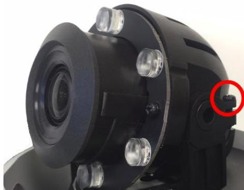
7. Install the dome lanyard if removed and then the dome cover and tighten the dome cover screws.
