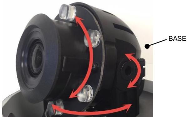
6. Tighten the locking screw to secure the camera module position.
