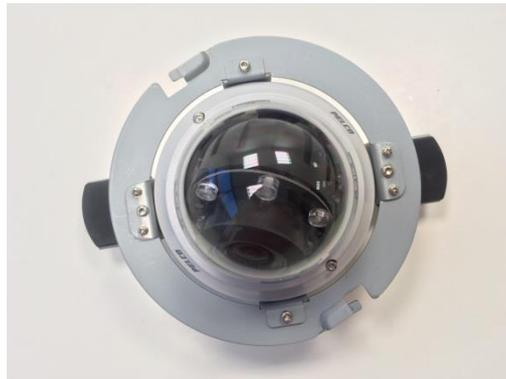
12. Put on the trim ring and rotate it clockwise to secure the trim ring on the bracket.
