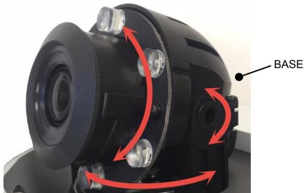
10. Tighten the locking screw to secure the camera module position.
