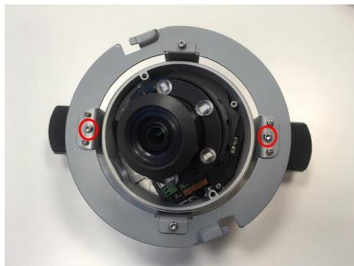
9. Adjust the angle of lens by pan and tilt. Grasp the base of the lens assembly to adjust.
