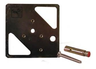
Mounting plate for a seismic detector. Weighs 0.27 kg (9.5 oz). Appropriate for mounting the seismic detector to steel or concrete surfaces. Screw or weld the mounting plate directly on an object.
