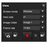
You can change the screen mode, size of the image, image codec mode and frame rate. Also, still images and movies can be saved (movie saving can also be stopped) from here.
