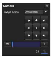
The camera control panel appears when **SolidPTZ** is set to **On**. This panel allows you to control the camera's pan/tilt/home position and zoom (page 17). In addition, you can obtain authority to operate the camera in exclusive control mode.
