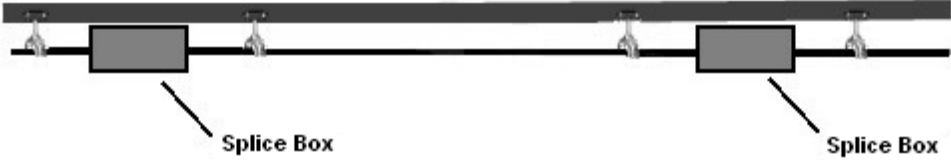
Splice box fixing
