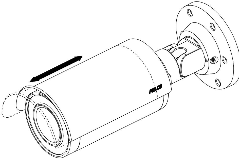
**FIGURE 2 - 9: ADJUSTING THE PROTECTION SHIELD HOOD**
