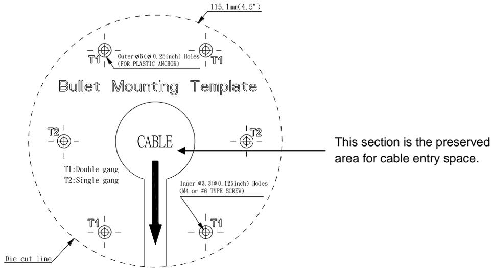
FIGURE 2 - 1: MOUNTING TEMPLATE
