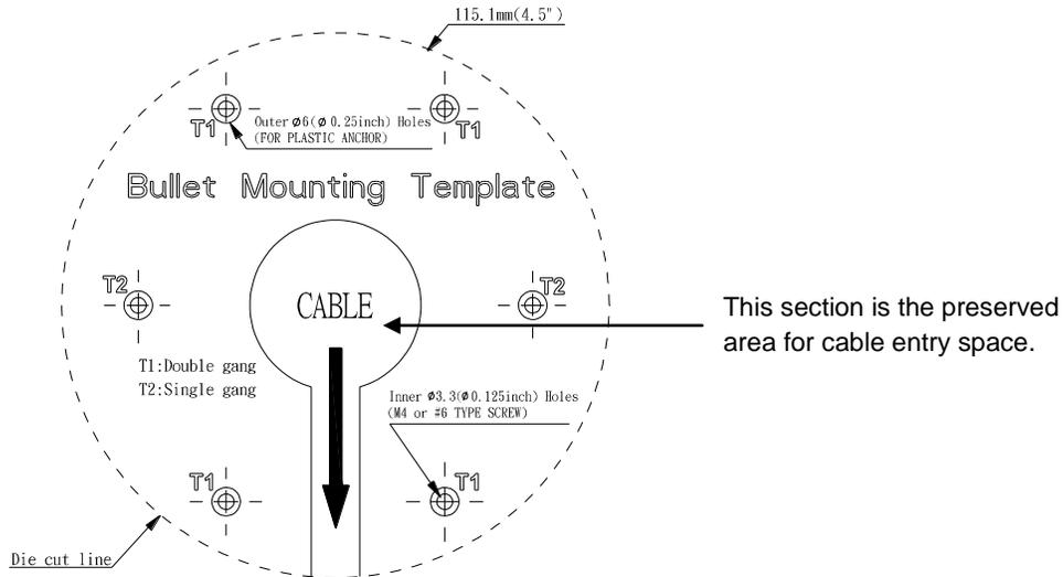
FIGURE 2 - 1: MOUNTING TEMPLATE
