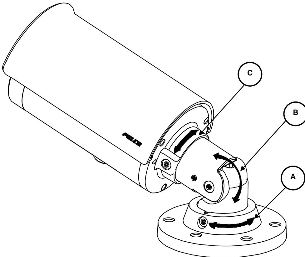
**FIGURE 2 - 8: ADJUSTING THE CAMERA POSITION**
